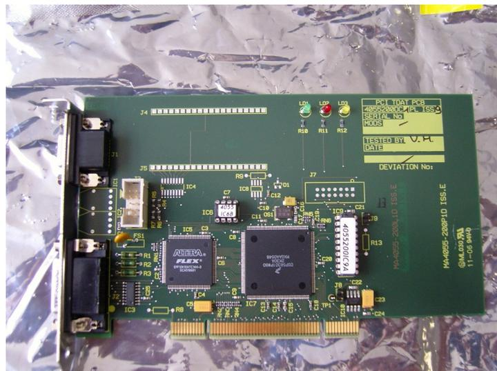
The PCI TDAT card was made for use in modern PCs. The bad thing is, that this card is not a true plug and play card and you need special software change notes. First you install Windows with standard PC drivers. You can change the settings in the device manager, click on the computer icon and change the driver from ACPI PC to
