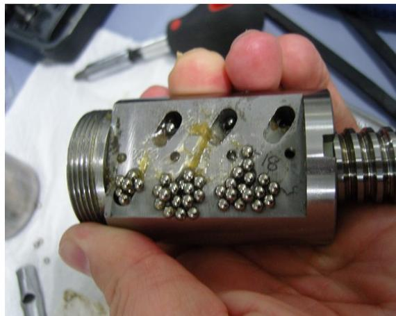
Figure 4: by turning the screw the balls move out
